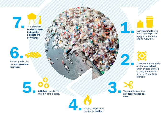
The sophisticated Recycled-Resource process produces a usable granulated feedstock from used plastic packaging. So what happens next? Furniture maker HOUE shows how it's done: with a designer chair made from recycled plastic packaging. While proving that climate protection and design are a great match.
